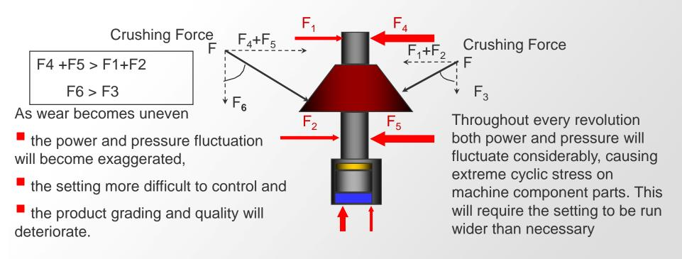
Zero reaction at any point during the revolution will suggest a portion of the chamber is empty
