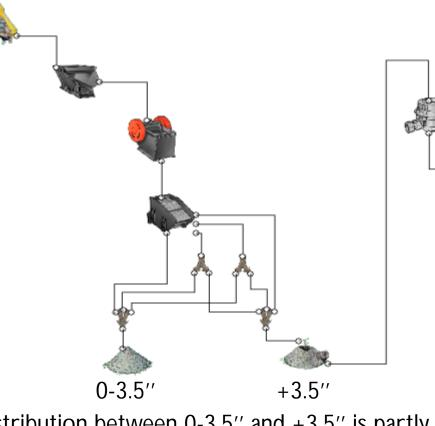
Distribution between 0-3.5" and +3.5" is partly controlled by the blasting result
