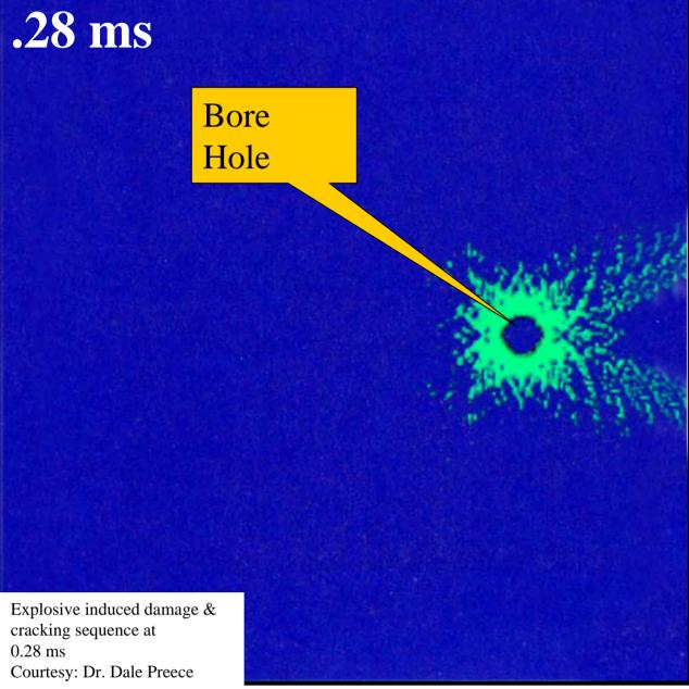
Cracking In Vicinity of Blast Hole
