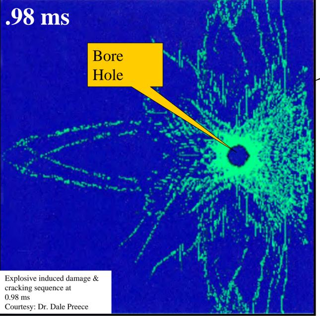
Cracking In Vicinity of Blast Hole
