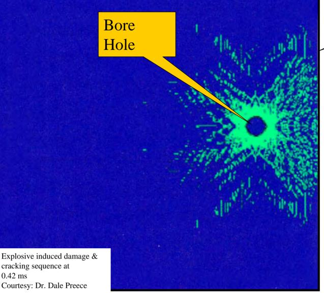
Cracking In Vicinity of Blast Hole
