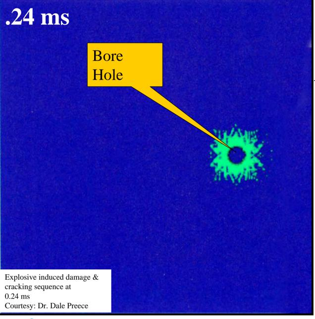
Cracking In Vicinity of Blast Hole
