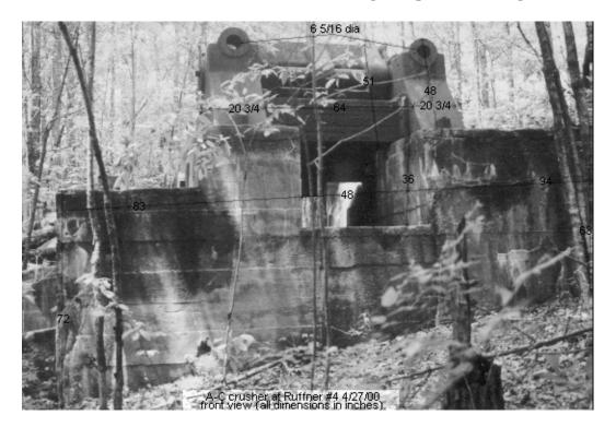
We have 2 extant crushers of the "coffee grinder" design on Ruffner. The remains of the gyratory cone crushers at mines #2 & #3 are quite similar to one which can be seen easily on Arkadelphia Road, at the corner of Wade Sand and Gravel, not far from I-59. The crusher at Ruffner #4 is entirely different, and thoroughly enticing. Note the wording on the stiffener beam. I had no idea what
