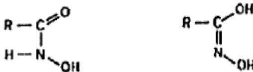
Figure 2.13: Tautomers of hydroxamic acid, hydroxyamide (left) and hydroxyoxime (right) (Pradip and Fuerstenau, 1983)
