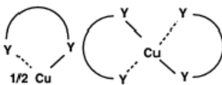
Figure 2.11- A chemisorbed chelating reagent on a copper oxide surface. Typical monolayer formation (Fuerstenau et al, 2000)
