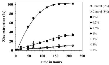
Figure 5. Effect of chloride on the extraction of zinc from the ore (1% w/v) by YTF1 strain at pH 1.6, 50°C and 0.02% w/v yeast extract
