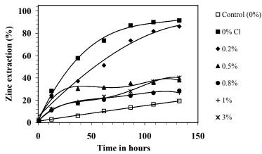
Figure 6. Effect of chloride on the extraction of zinc from the ore (1% w/v) by THWX strain at pH 1.6, 50oC and 0.02% w/v yeast extract
