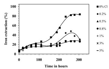
Figure 4. Effect of chloride on the extraction of iron from the ore (1% w/v) by DSM 583 strain at pH 1.6 and  $30^{\circ}$ C
