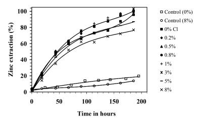
Figure 8. Effect of chloride on the extraction of zinc from the ore (1% w/v) by DSM 1651 strain at pH 1.4 and 70°C
