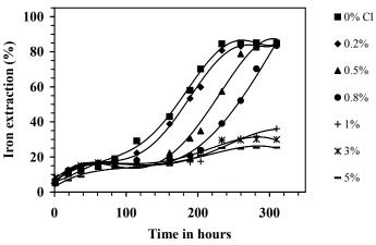
Figure 2. Effect of chloride on the extraction of iron from the ore (1% w/v) by WJM strain at pH 1.6 and  $30^{\circ}$ C
