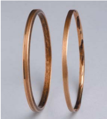
FIGURE 7: Oil rings in as-new ("wide and chamfered") condition on left, and abraded (i.e., badly worn and now without chamfer) condition on the right side. Record both before versus after widths ( Highlight 9 , also Refs. 1 and 4)
