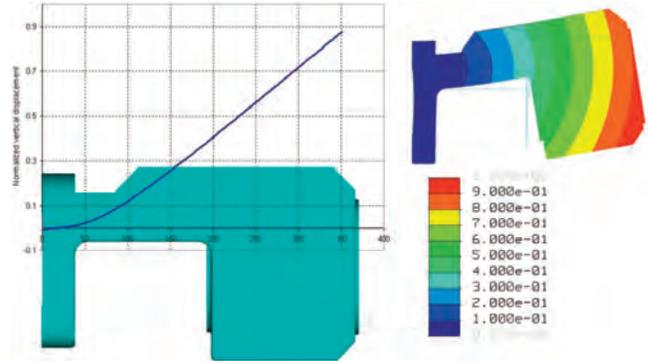
Figure 13. Bearing Housing Vertical First Modal Shape Displacements.
