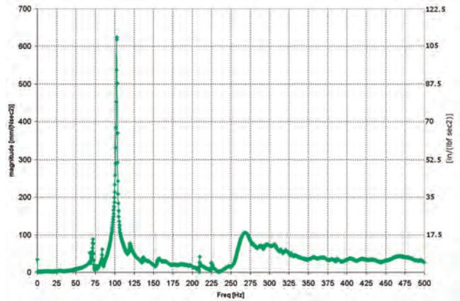
Figure 17. New Design Bearing Housing Response Function Magnitude.
