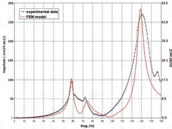
Figure 10. Comparison Between Calculated Frequency Response and Experimental Data for Drive and Horizontal Direction.
