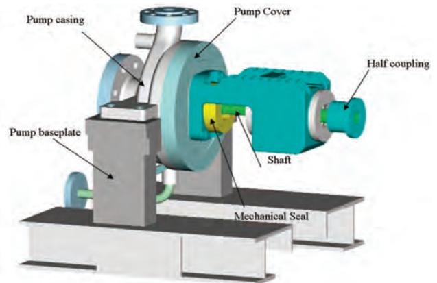
Figure 1. Typical View of the OH2 Type Pumps That Were Studied.
