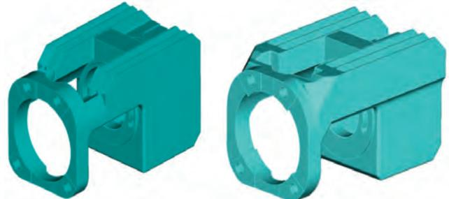
Figure 14. Comparison Between the Original (Left) and the Optimized Bearing Housing (Right).
