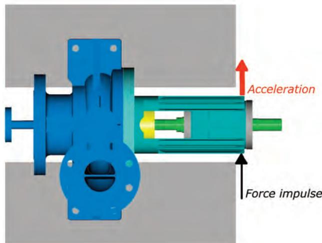
Figure 4. Drive End Impulse/Measurement Location in Horizontal Direction.
