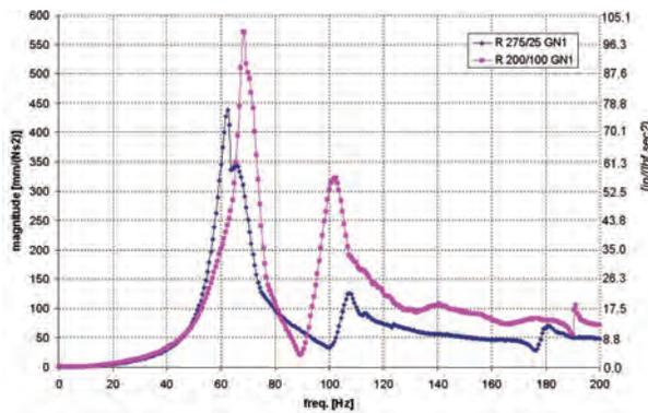
Figure 7. Comparison of Drive End Vertical Direction Frequency Response Magnitude for Two Different Pump Configurations Equipped with the Same Bearing Housing.
