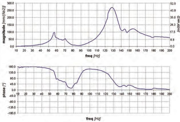
Figure 6. Drive End Frequency Response Magnitude and Phase, Horizontal Direction.
