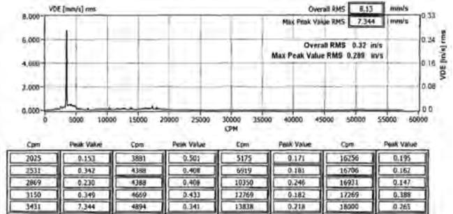
Figure 18. Velocity Vibration Value (RMS) Measured at Drive End Position in Vertical Direction, Original Housing Design.
