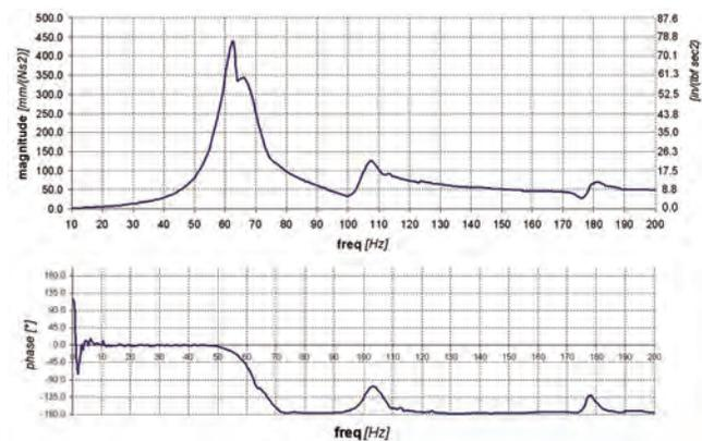
Figure 5. Drive End Frequency Response Magnitude and Phase, Vertical Direction.
