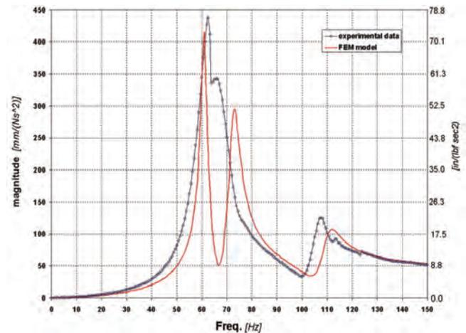
Figure 9. Comparison Between Calculated Frequency Response and Experimental Data for Drive and Vertical Direction.
