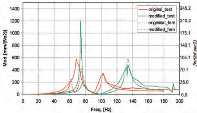
Figure 15. Drive End Frequency Response for Original and Modified Bearing Housing.
