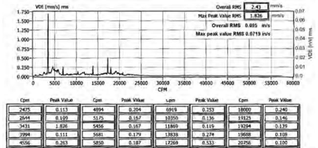
Figure 19. Velocity Vibration Value (RMS) Measured at Drive End Position in Vertical Direction, Improved Housing Design.
