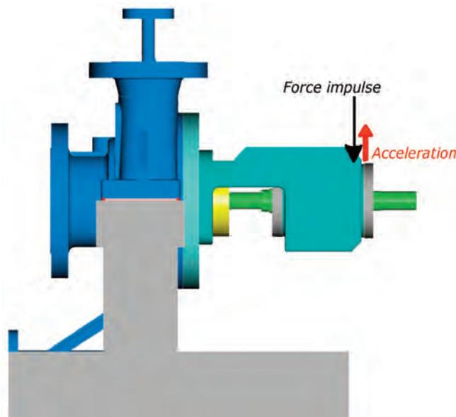
Figure 3. Drive End Impulse/Measurement Location in Vertical Direction.
