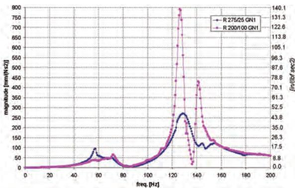
Figure 8. Comparison of Drive End Horizontal Direction Frequency Response Magnitude for Two Different Pump Configurations Equipped with the Same Bearing Housing.
