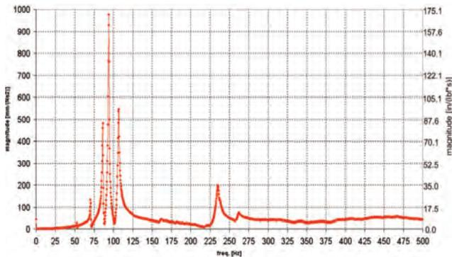
Figure 16. New Design Bearing Housing Frequency Response Magnitude.
