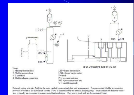
Figure D.16 — Standard seal flush Plan 53B
