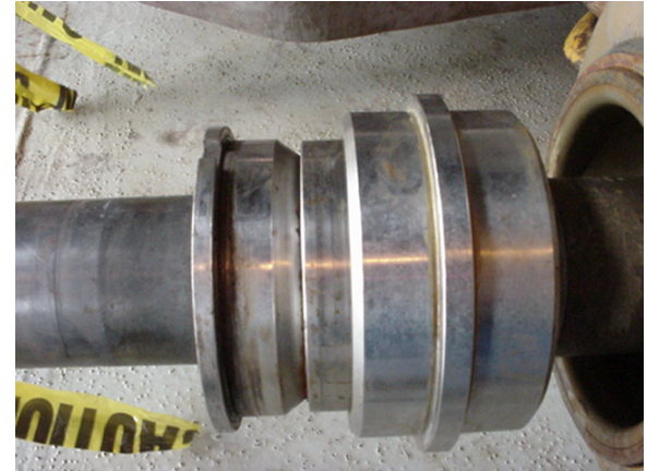
Throttle sleeve pushed off the fit and welded to throat
