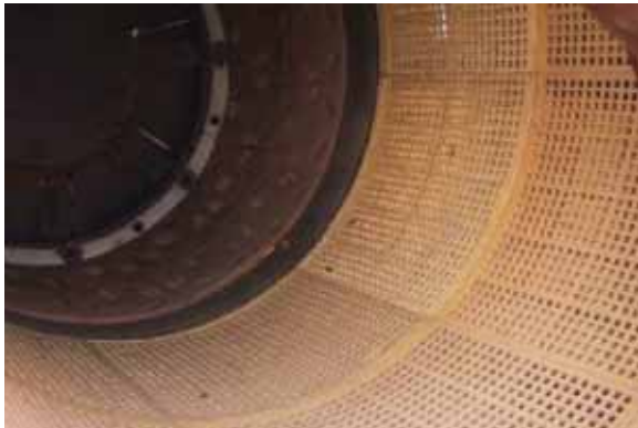
Trommel screen separates particles discharged from the mill
