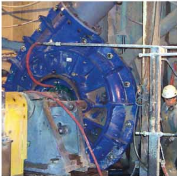
Warman 450 MCR elastomer lined mill circuit pump on SAG mill service
