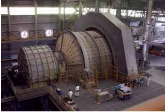
Typical SAG mill in a copper treatment plant
