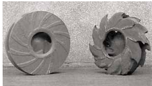
New Warman mill circuit pump impeller compared to a worn impeller after pumping 5 million tons of ore. The worn impeller efficiency had reduced by just 3 percent during its wear life
