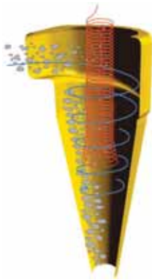
Internal profile of the Cavex hydrocyclone illustrating the effects of the full circle, three dimensional curvature
