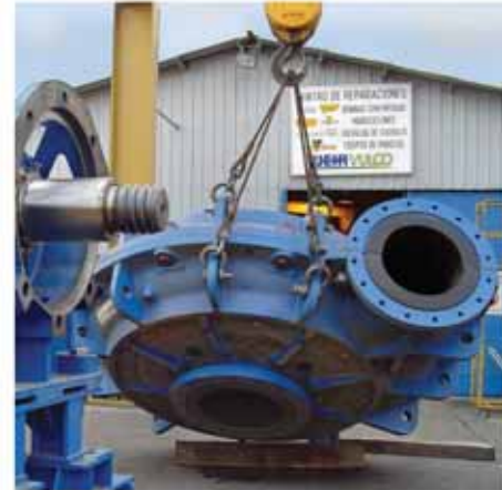
Above: A new innovative quick change device has been developed for faster removal of the larger MC range pump wet ends. A 650 MCR wet end being removed in Santiago, Chile
