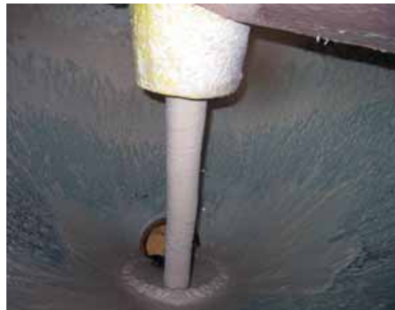
Rope flow pattern from a spigot with a diameter which is too small
