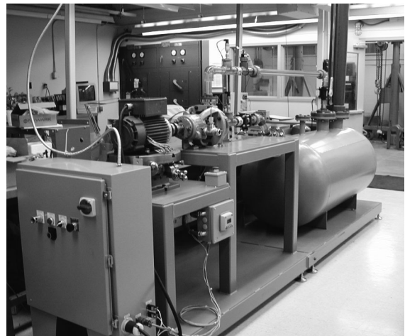
Figure 2. Intelligent Motor-Pump-Controller Demonstration System.
