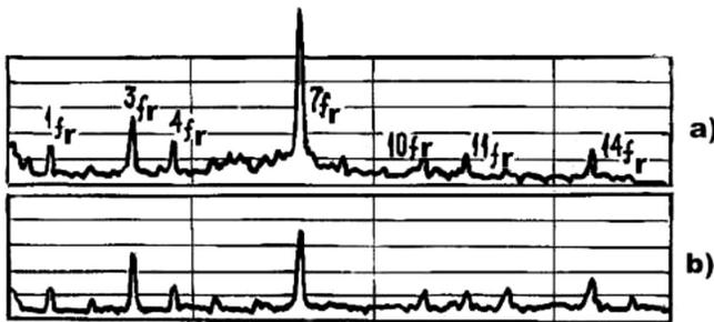
Figure 2. Spectra of Pressure Pulsations in the Volute (Above) and in the Diffuser Vane Channel (Below) of a Centrifugal Pump.
