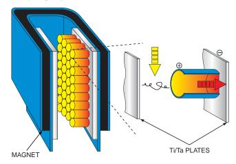
Ion pumps are the primary choice for all true UHV chambers. They are clean, bakeable, vibration-free, operate from  $10^6$  Torr to  $10^{-11}$  Torr with low power consumption, and have long operating lives. All ion pumps have the same basic components: a parallel array of short, stainless steel tubes, two plates (Ti or Ta)
