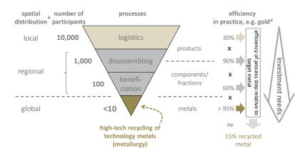
**Figure 13.** Process chain of recycling for consumer goods: technology metals from printed circuit boards [60].
