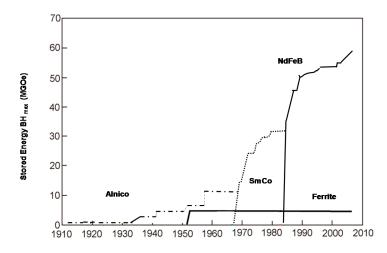
**Figure 11.** Development of permanent magnets, modified from [48]. The *y*-axis is the magnet performance, expressed as stored energy (BH)<sub>max</sub>, measured in units of megagauss-oersted (MGOe).
