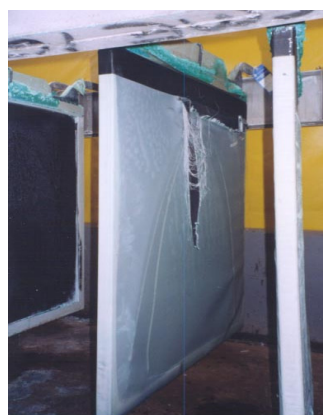
Figure 11 – Damaged Anode Bag
