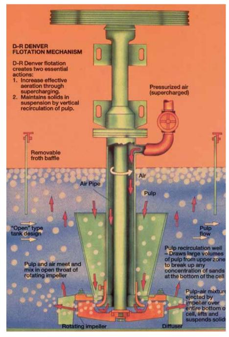
the impeller into the cell creating a homogenous mixture in the tank. The action is possible only in flotation machines with "top feed" impellers such as used on Metsos DR flotation machines.
