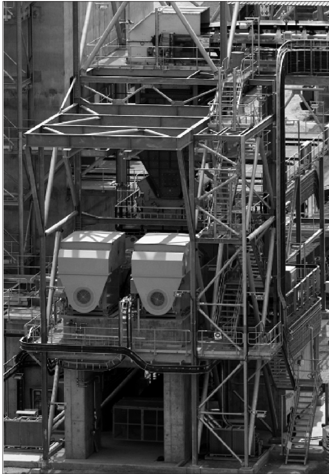
Figure 5. HPGR Polycom 22/16- 8 at Mogalakwena plant
