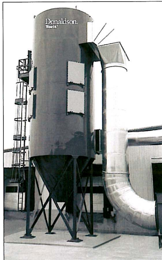
RF Baghouse Collector
