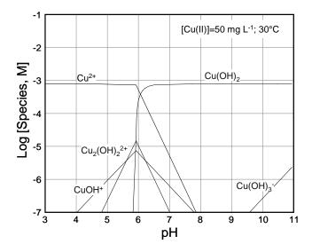
**Fig. (2).** Species distribution diagram of the Cu(II)-H<sub>2</sub>O system at 25°C for a Cu(II) concentration of 50 mg/L, showing the predominance of Cu<sup>2+</sup> at pH below 6 and the predominance of Cu(OH)<sub>2</sub> above this pH (HSC Chemistry v. 5.11).
