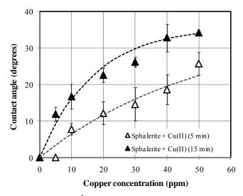
**Fig. (3).** Effect of  $Cu^{2+}$  concentration and conditioning time on the contact angle of sphalerite. The tests were carried out at 30°C, natural pH (5.4) and 10<sup>-3</sup> M NaNO<sub>3</sub> ionic strength; the contact angle was measured at pH 10. The dotted lines were obtained with Equation (9), developed in this work.
