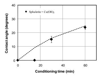
**Fig. (7).** Effect of conditioning time on the development of the hydrophobic character of sphalerite activated with 5 mg/L Cu(II) in the form of Cu(OH)<sub>2</sub>. The dotted line was obtained with Equation (9).
