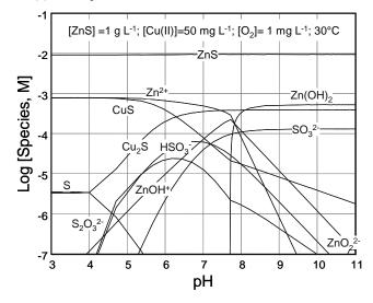
**Fig. (4).** Species distribution diagram for the activation of ZnS with Cu(II) at 30°C, when considering a solution relatively free of dissolved oxygen and the metastable products of the oxidation of sulphide [5]. HSC Chemistry v. 5.11.
