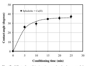
**Fig. (5).** Effect of conditioning time on the development of the hydrophobic properties of sphalerite. The tests were carried out at  $30^{\circ}$ C and  $10^{-3}$  M NaNO<sub>3</sub>. Conditioning was performed at natural pH (5.4), and the contact angle was measured at pH 10. The dotted line was obtained with Equation (9).
