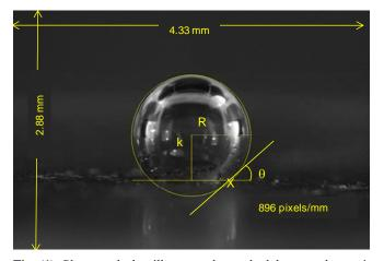
Fig. (1). Photograph that illustrates the methodology used to estimate the slope to the circle in the point of the three-phase contact (x).
