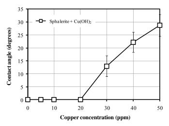
**Fig. (6).** Effect of Cu (II) concentration as Cu(OH)<sub>2</sub>, on the contact angle of sphalerite as a function of conditioning time. The tests were carried out at  $30^{\circ}$ C, pH 9 and  $10^{-3}$  M NaNO<sub>3</sub> ionic strength.
