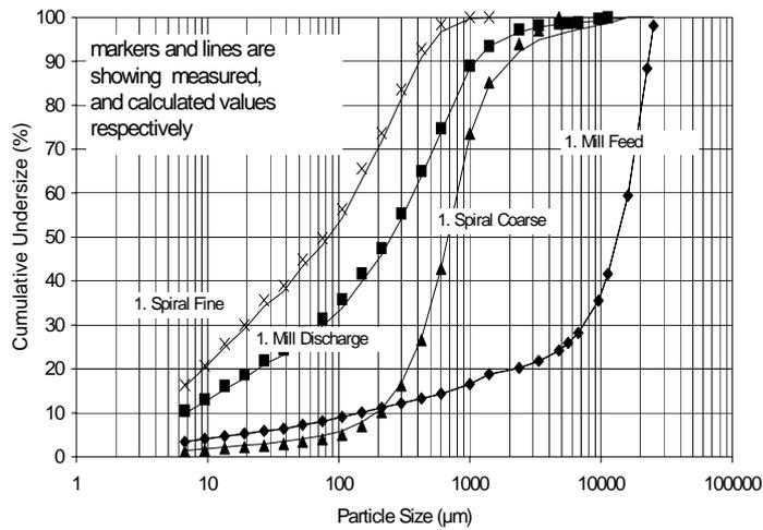
Fig. 4. Measured and mass balanced values around 1<sup>st</sup>, 2<sup>nd</sup> primary grinding circuit
