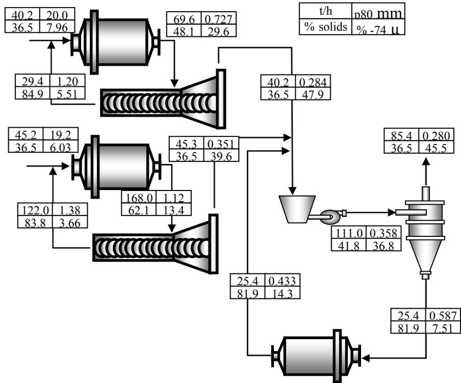
Fig. 3. Flow rates after mass balancing
