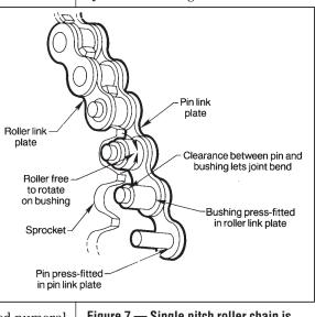
Figure 7 — Single pitch roller chain is available in pitch sizes above 3/8 in. Single and multiple-strand versions are available.
