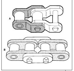
Figure 11 — Heavy duty, offset sidebar engineering steel roller chain, A, and heavy duty, straight sidebar roller type conveyor chain, B.
