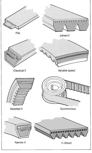
Figure 1 — Representative belt configurations.
