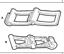
Figure 10 — Pressed steel detachable link chain, A, and malleable iron detachable link chain, B.
