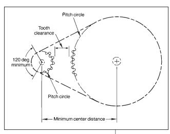
7. Center distance between shafts. (If distance is adjustable, what is the range of adjustment?)
