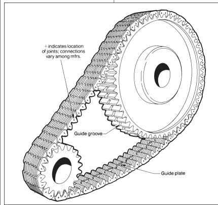
Figure 9 — Inverted tooth (silent) chain drive. These sprockets are grooved for center quide chain.
