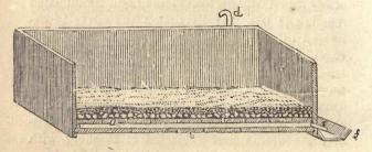
The boxes must be made as water-tight as possible and provided with a filter at the bottom. The filter is prepared in two ways, either as represented in Fig. 10 by fixing a false bottom, a, provided
