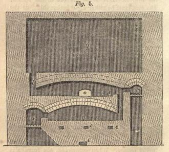
in Fig. 5, in longitudinal cross section. The lower hearth, a, is nine feet long and ten feet wide. The
