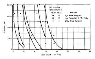
Figure 12.—Tungsten carbide case depth versus pressure for hot pressing tungsten powder at 1500° and 1800° C. (83)
