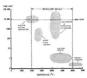
Figure 2.—High-temperature materials requirements. (17)
