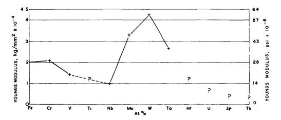
Figure 3.—Structural continuity in 6cc metals (upper) and the corresponding Young's modulus (lower), illustrating the relative position of tungsten in the series. (18)
