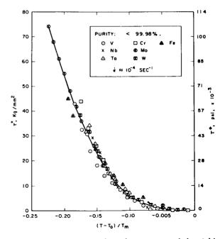
Figure 5.—Correlation of thermal component of the yield (stress  $\tau^*$  with the parameter  $(T-T_o)/T_m$  for the bcc metals. (28)
