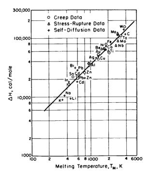
Figure 4.—Correlation of the activation energies for creep, stress-rupture, and self-diffusion with the melting temperature. (20)
