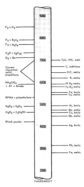
Figure 1.—Combustion temperatures of rocket propellants plotted against the melting and vaporizing temperatures of various component materials. (16)
