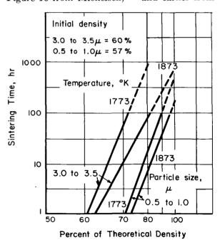
Figure 16.—Sintering rates of porous-tungsten ionizers.
