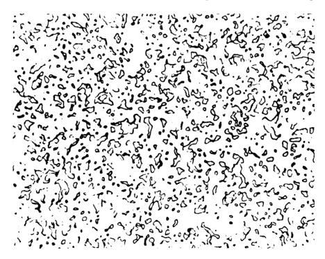
Figure 13.—This photomicrograph, taken at 500 × from an unetched specimen, shows the silver evenly dispersed throughout the tungsten matrix.
