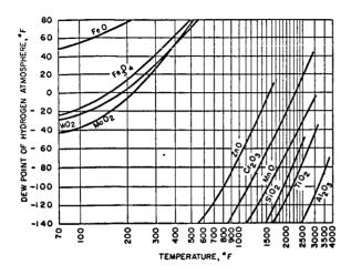
Figure 6.—Metal-metal oxide equilibria in hydrogen atmospheres. (35)
