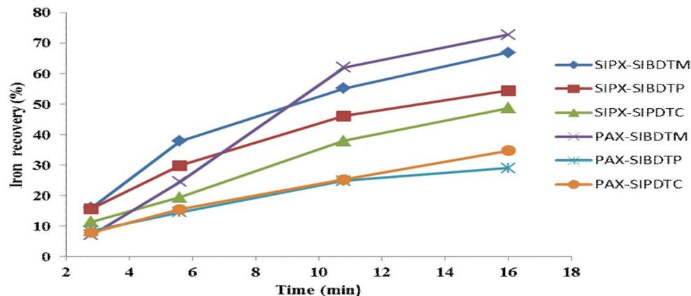
Fig. 7. Fe recovery as a function of floatation time by using the mixture of collectors
