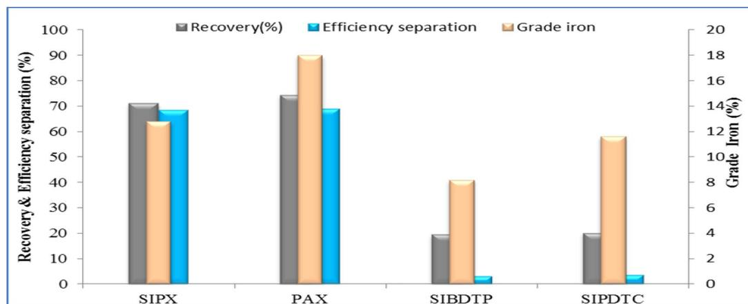
Fig.2. The results of Fe metallurgy calculations in the presence of pure collectors
