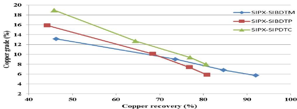
Fig.4. Cu grade as a function of recovery by using the mixture of SIPX with other collectors.
