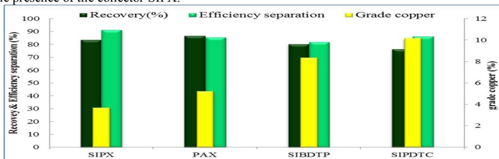
**Fig.1.** The results of Cu metallurgy calculations in the presence of pure collectors
