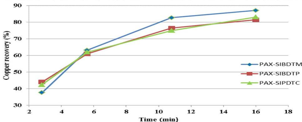
Figure 5. Cu recovery as a function of flotation time by using the mixture of PAX with other collectors.
