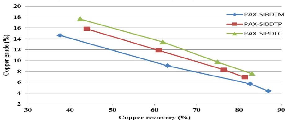
Fig.6. Cu grade as a function of recovery by using the mixture of PAX with other collectors.
