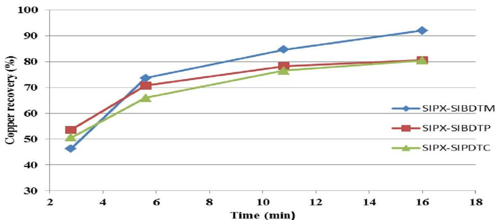
Fig.3. Cu recovery as a function of floatation time by using the mixture of SIPX with other collectors.
