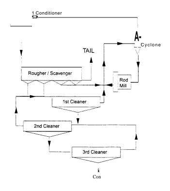
FIG 3 - Lead flotation circuit.
