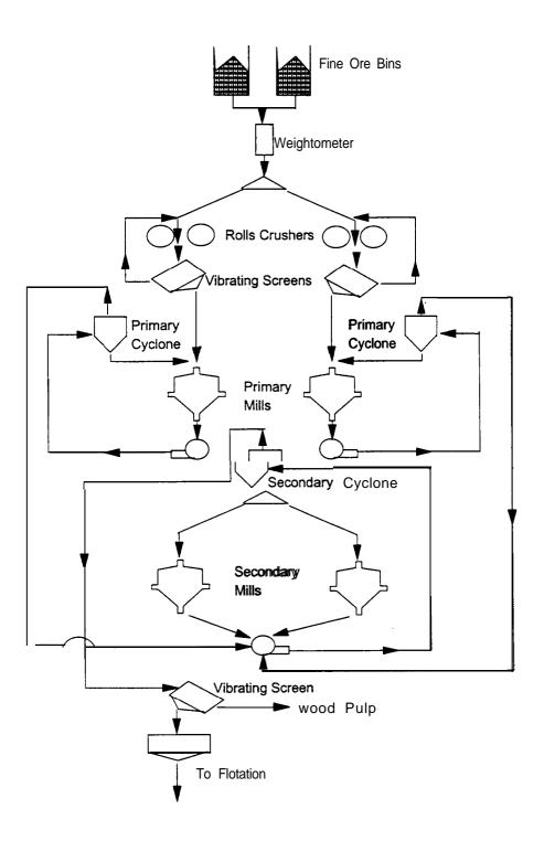
FIG 1 - Grinding circuit flowsheet.
