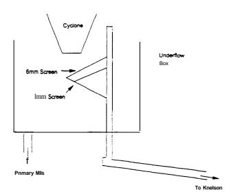
FIG  $8 \cdot \text{Cyclone}$  underflow screen / cutter.
