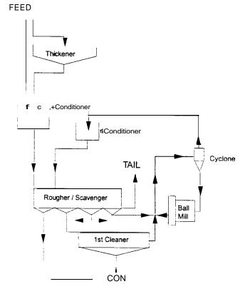
FIG 4 - Zinc flotation circuit.
