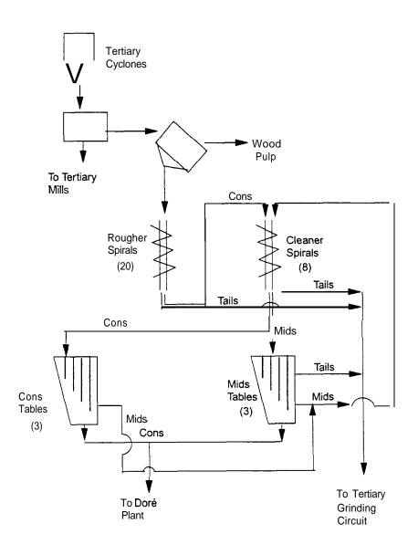
FIG 5 - Gravity plant flowsheet.
