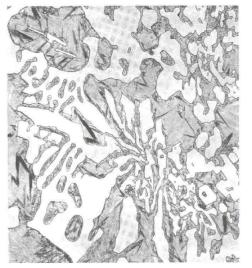
Typical microstructure of class 1 type D nickel-chromium white cast iron.
