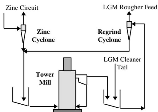
**Figure 1. Hilton Tower mill regrind circuit**
