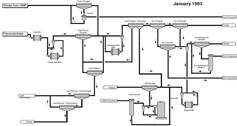
Figure 2. Flowsheet after the installation of increased grinding and flotation capacity- After Young et al, 1997
