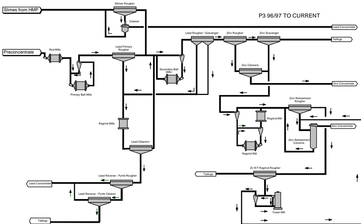
Figure 3 - Current flowsheet after the installation of regrinding of lead rougher and zinc concentrate
