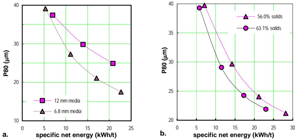
Figure 4: Media size (a) and slurry % solids (b) effect on pilot Tower mill efficiency (Jankovic, 1998)
