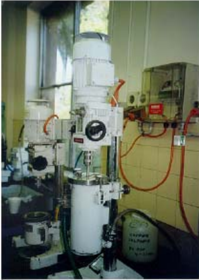
Figure 2. The 1.5-litre Netzsch batch mill.
