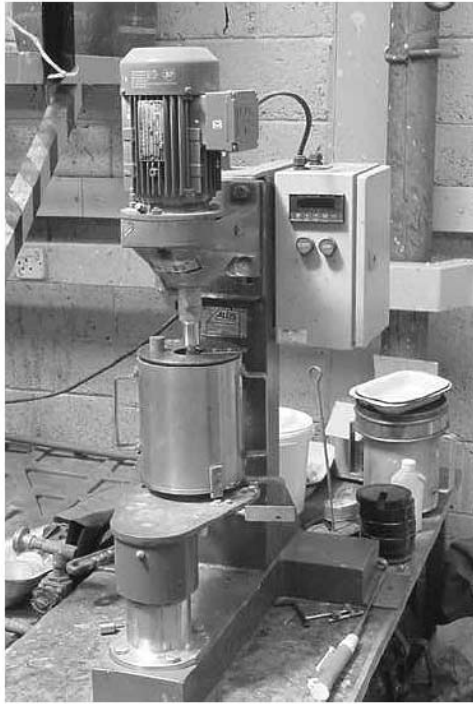
Figure 16. Laboratory and industrial size STIRRED MEDIA DETRITOR (SMD®)
