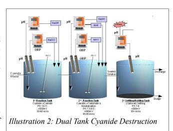
In the first tank, conditions are adjusted to oxidize
