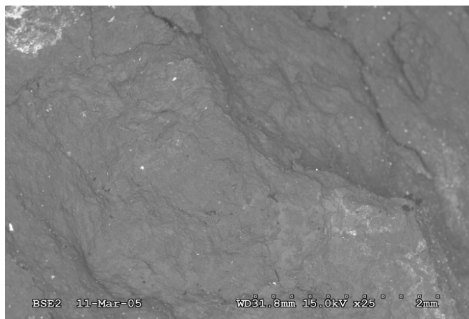
Figure 9. Scanning electron microscope backscattered electron image of a fractured leached ore particle surface after impregnation with lead nitrate to highlight pore areas in white.
