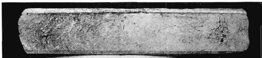
FIG. 4.—SLAB MADE AND PHOTOGRAPHED AT NORWAY STEEL & IRON CO.'S WORKS. PLATE STEEL ROLLED ONE WAY FROM 13 BY 22 IN. TO 4 BY 22 IN. EXCELLENT SLAB. BLOWHOLES VERY FAR IN. MADE IN 1884.
