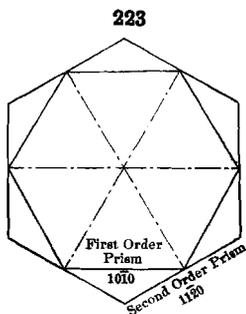
The relation in position between the first order prism (and pyramids) on the one hand and the second order prism (and pyramids) on the other will be understood better from Fig. 223, representing a cross section of the two prisms parallel to the base *c*.
