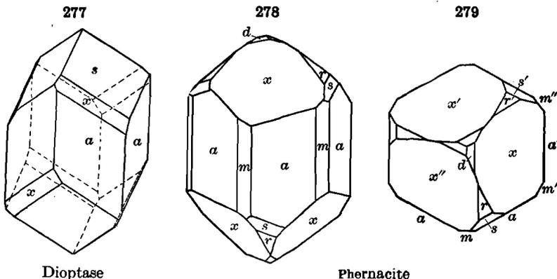
projections of a crystal of phenacite with the following forms: first order prism,  $m(10\bar{1}0)$ ; second order prism,  $a(11\bar{2}0)$ ; third order rhombohedrons,  $x(12\bar{3}2)$  and  $s(21\bar{3}1)$ ; first order rhombohedrons,  $r(10\bar{1}1)$  and  $d(01\bar{1}2)$ .
