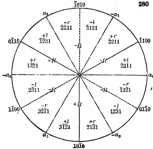
shows the distribution of the faces of the four rhombohedrons of the third order (+r, +l, -r, -l) relatively to the faces of the unit hexagonal prism (1010).
