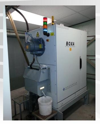
XRF Measurement of Slurry
