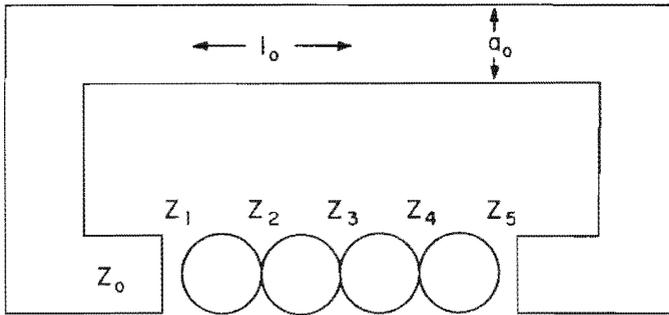
FIGURE 5. - Magnetic Circuit of Separator.
