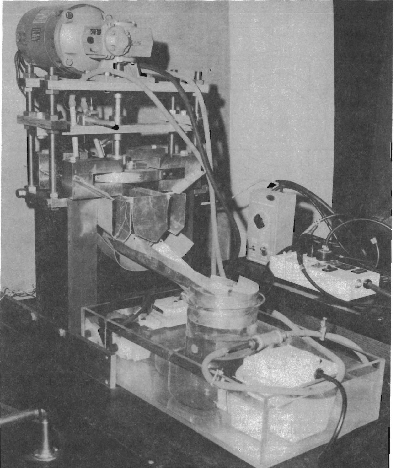
FIGURE 3. - Complete Separator With the Mechanical Drive Above the Matrix and the Magnetizing Coil Below the Discharge Launderers.
