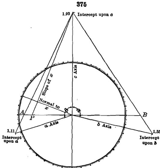
through the points  $A$  and  $B$  on the horizontal projections of the  $a$  and  $b$  axes. With the known angles  $\beta$  and  $\alpha$  it is possible to construct the  $a$  and  $b$  axes with their proper angular relations to the  $c$  axis. The intercepts of the face upon these two axes will be given by the extension of the lines from the point 1.93 on the  $c$  axis to the points  $A$  and  $B$ . In this way the intercepts of the face upon the three axes were obtained as 1.11a, 1.55b,
