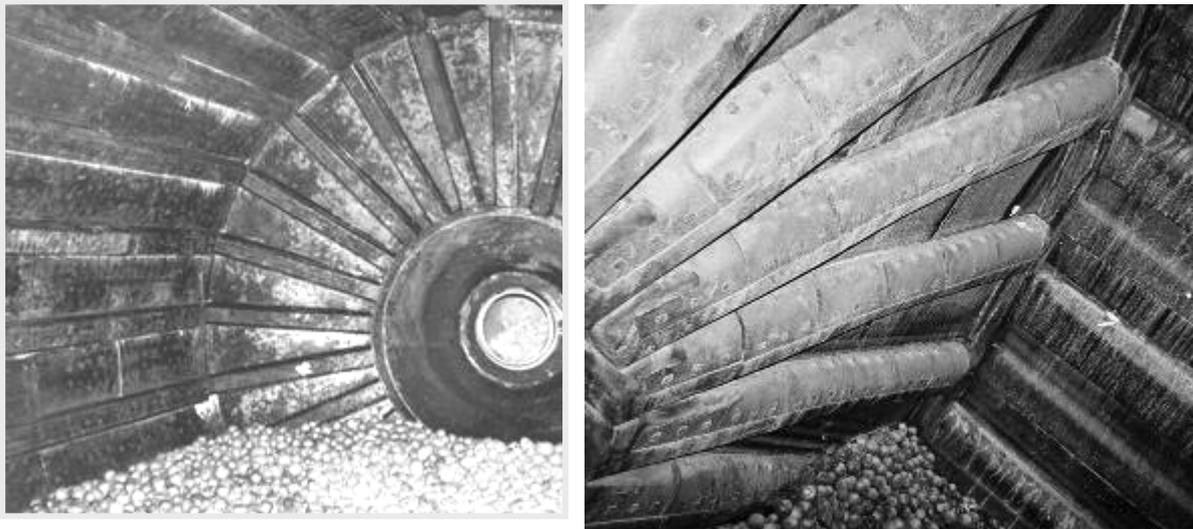
**Figure 6. Rubber lining in a ball mill and feed head metal capped lifter**
