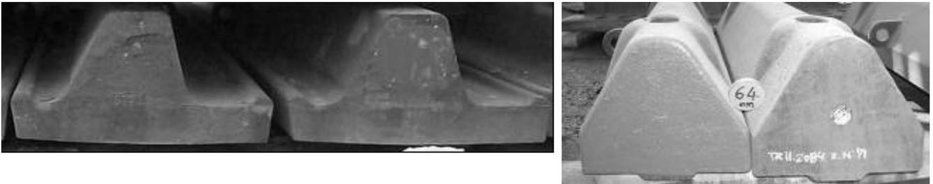
**Figure 4. Single Direction Top Hat Liners – integral liner, and bi-directional liners – removable lifters**
