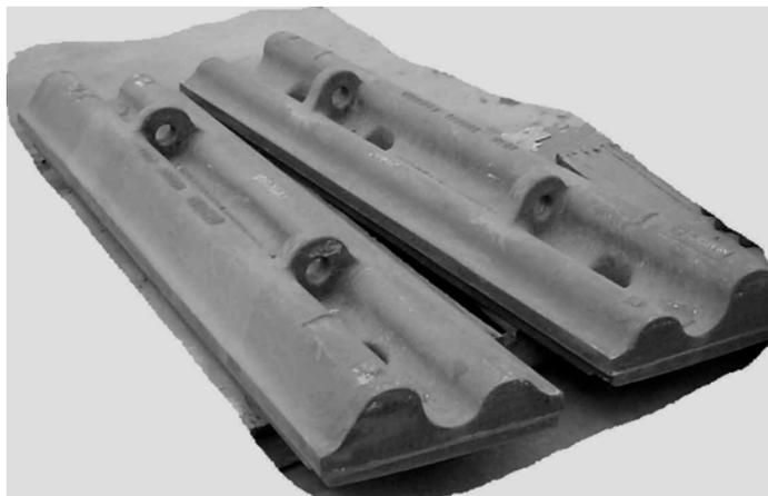
**Figure 5. High-low wave ball mill liner**
