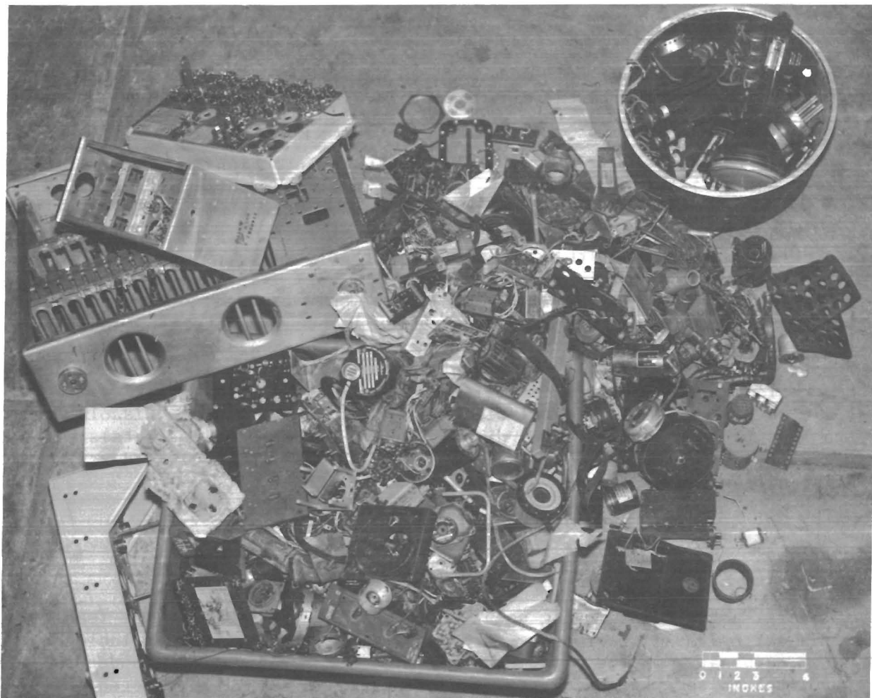
FIGURE 1. - Typical Military Electronic Scrap.
