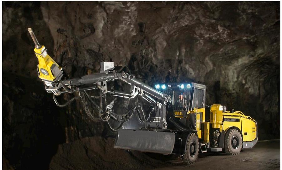
*Mechanized scaling with hydraulic hammer.*
