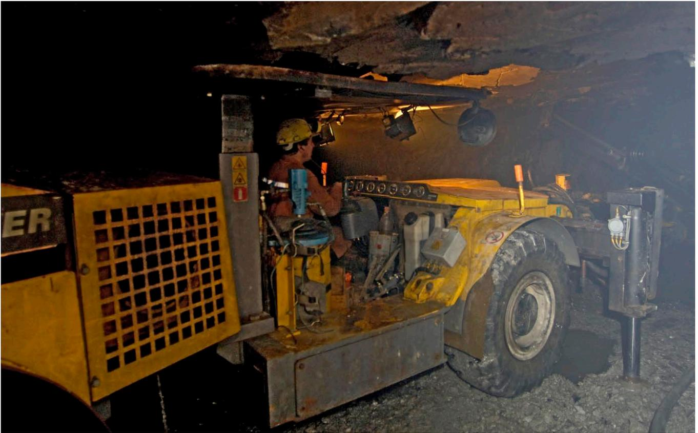
*Boomer S1 L drill rig in operation.*
