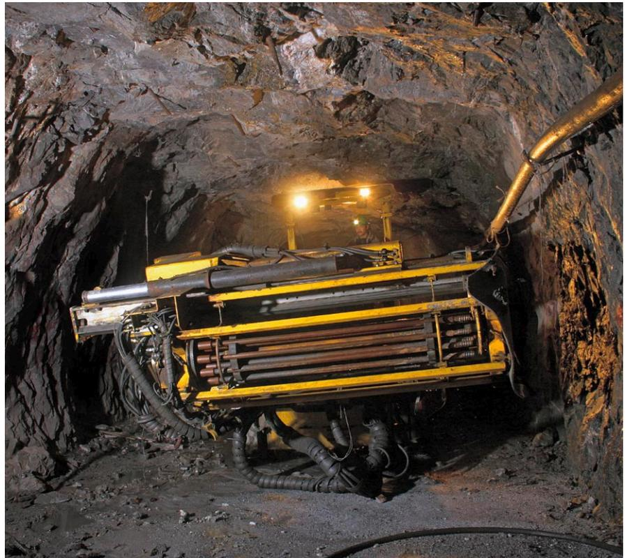
Setting up Simba 1254 for blast hole drilling.
