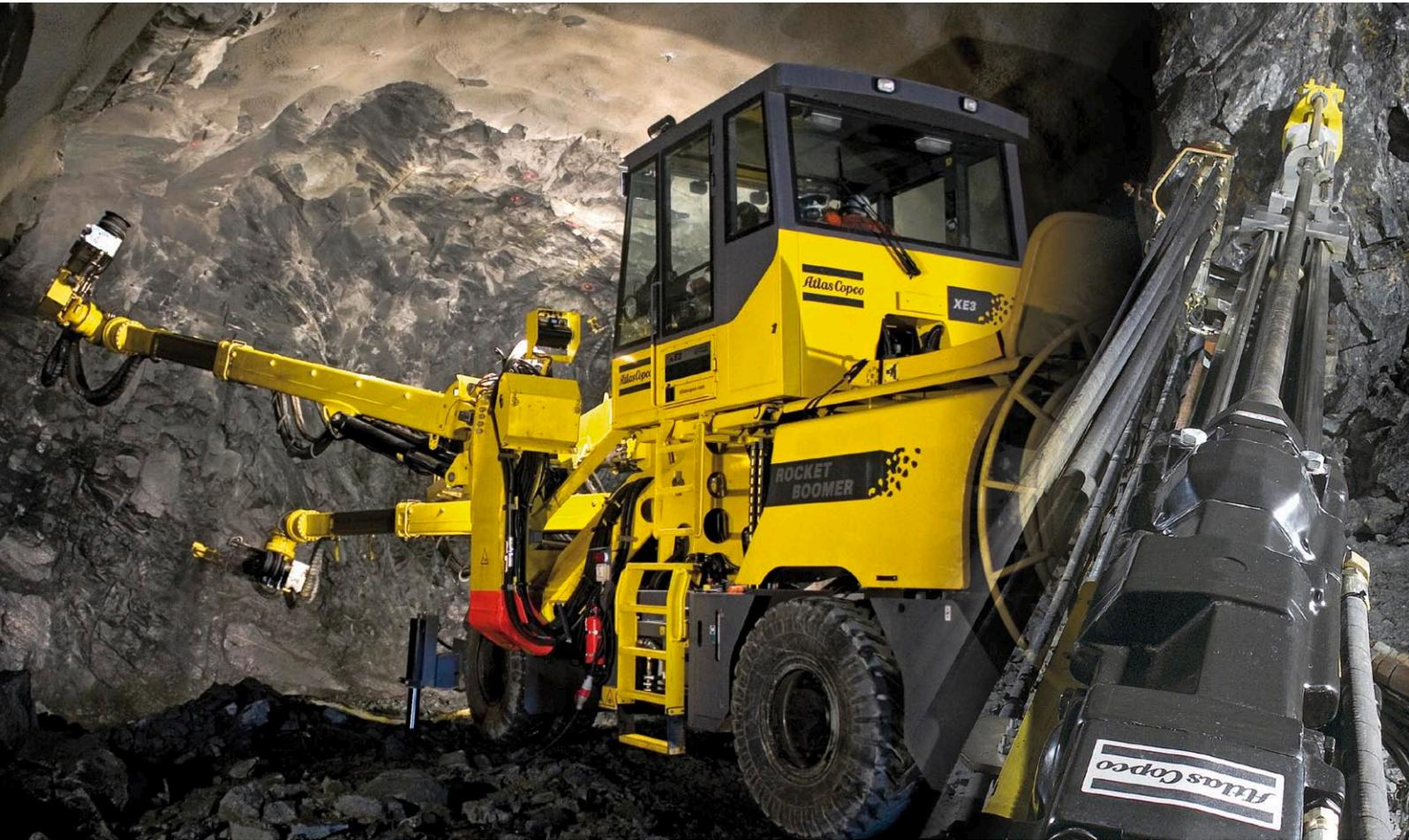
The Rocket Boomer E-series. A new face drilling rig that features the super-fast, prize-winning COP 3038 rock drill. It also introduces the BUT 45, a superb new boom that reduces hole deviation, provides extra large coverage area and slashes positioning time between holes by 50%. The result?
