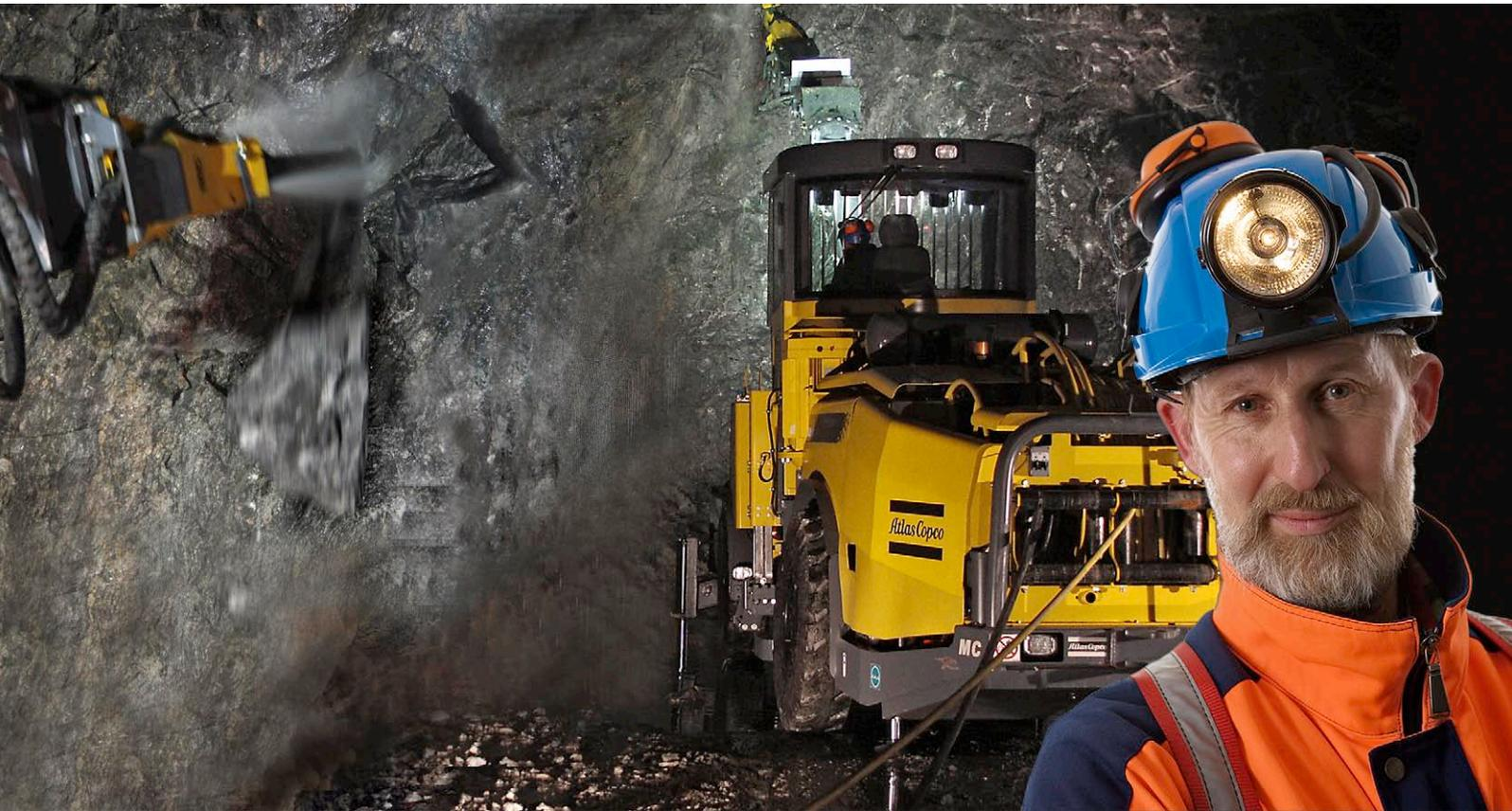
Add a solid body hydraulic breaker to a proven folding boom on the world's most tested underground carrier, and you have the Scaletec MC – a scaling rig for tunnelling and mining applications. Scaletec MC will give you higher productivity, less accidents, and take you a giant step along the route towards full mechanization.
