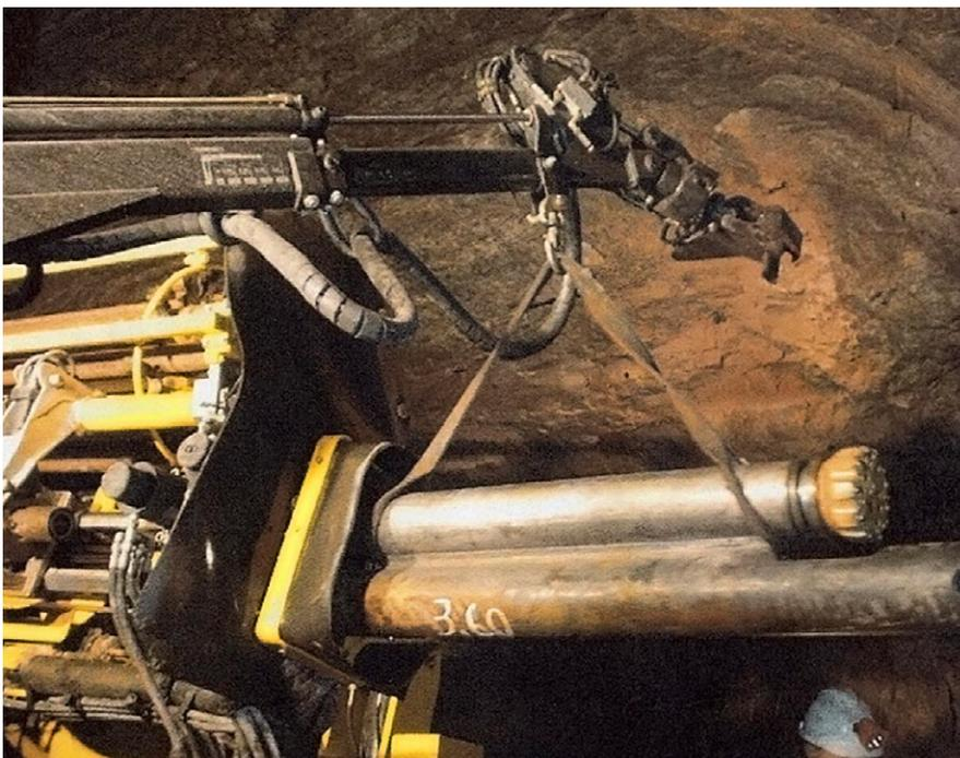
space for consecutive blasting. The drilling and blasting results are shown below. Hole opening, or downreaming, using a small-diameter reamer to enlarge an existing pilot hole, can also be carried out by an RBM.
