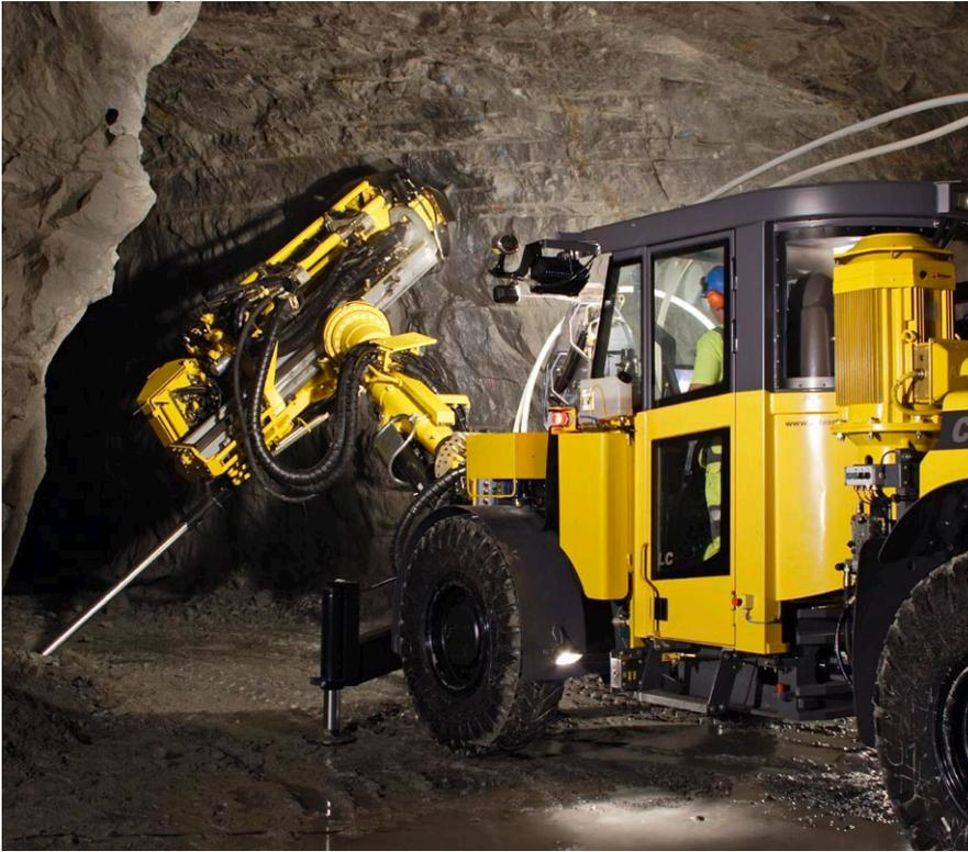
Mechanized cablebolting with Cabletec LC.
