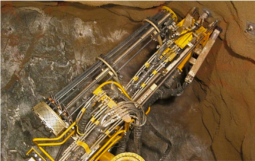
*Boltec LC installing Swellex Mn12 rockbolts.*
