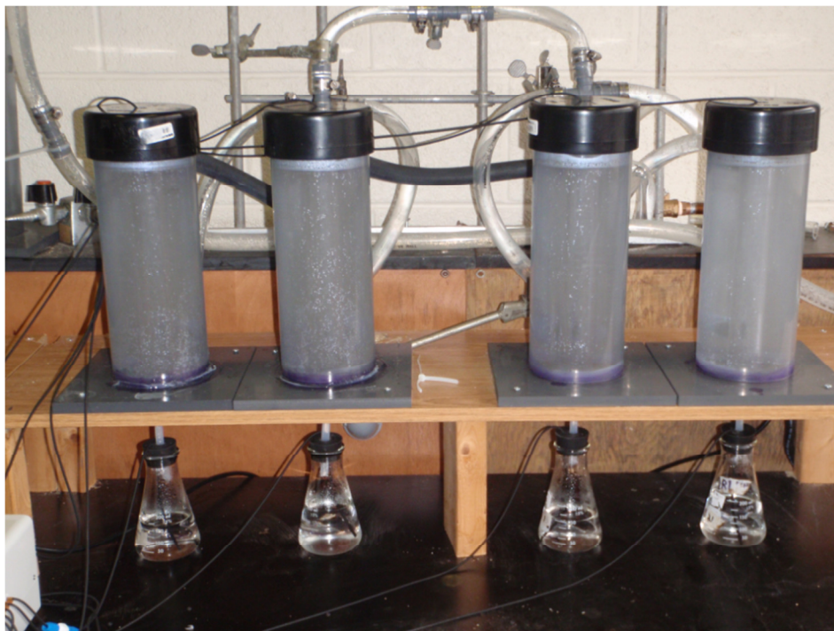
Figure 3.6: Miniature Leaching Column Apparatus Setup
