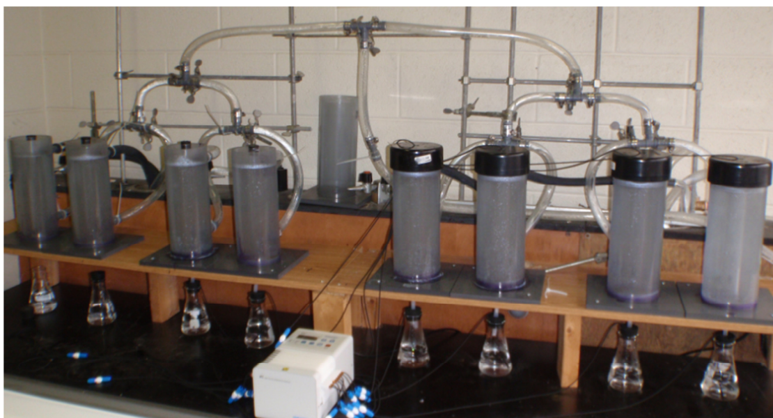
Figure 3.7: Miniature Leaching Column Apparatus Full Setup
