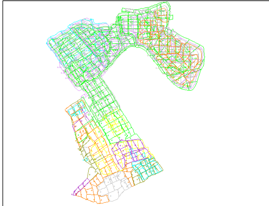
Figure 5 - Resulting Import of AutoCAD DXF file Into A METSIM Heap Leach Model
